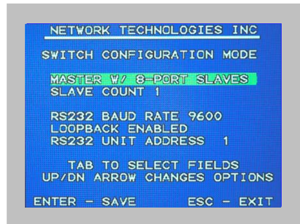
Figure 20- Switch configured as a master with one slave attached
